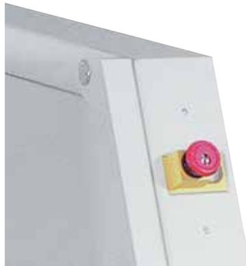
Prominent emergency-stop switch permits fast shredder shut-down
