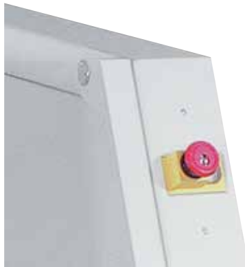
Prominent emergency-stop switch permits fast shredder shut-down
